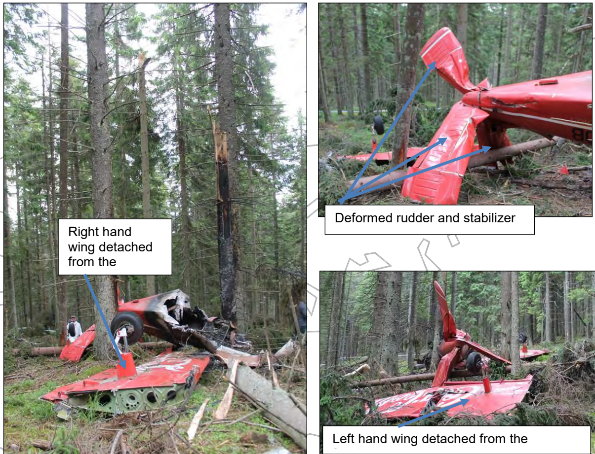
Fig. 11 – Deformations suffered by the aircraft upon impact with the firs/ground
