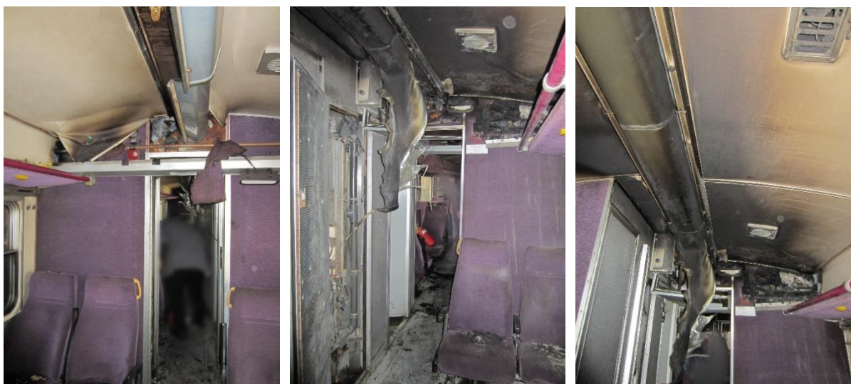
Fig.4.1.1.2: The appearance of passenger compartment DMK 710-004 on fire
