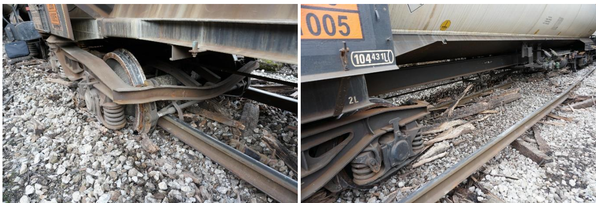
Figure 3.1.2: The appearance of the derailed wagon parts
