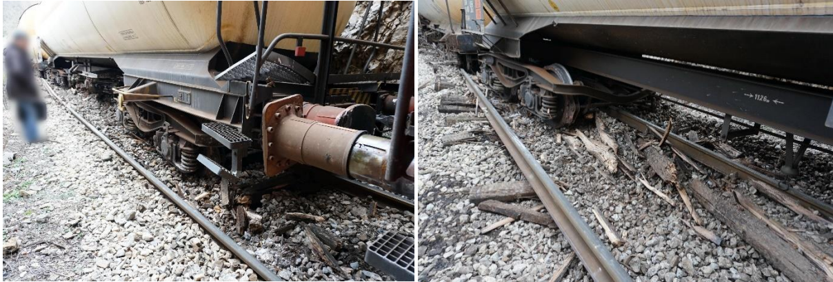
Figure 3.1.3: The appearance of the derailed wagon parts
