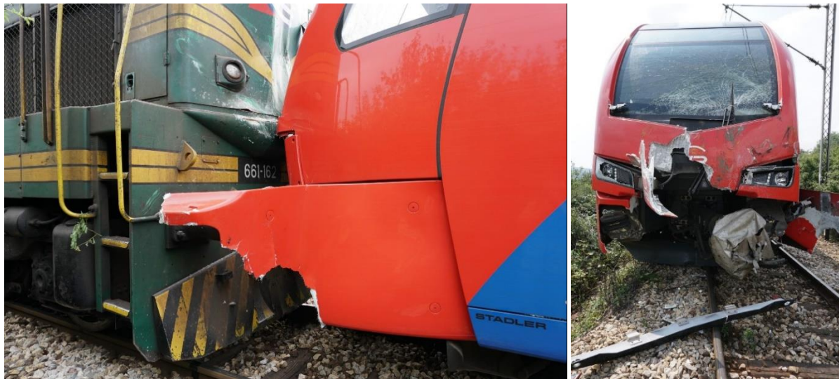
Fig. 4.3.1.1: The appearance of damages on the railway vehicles after the collision of trains
