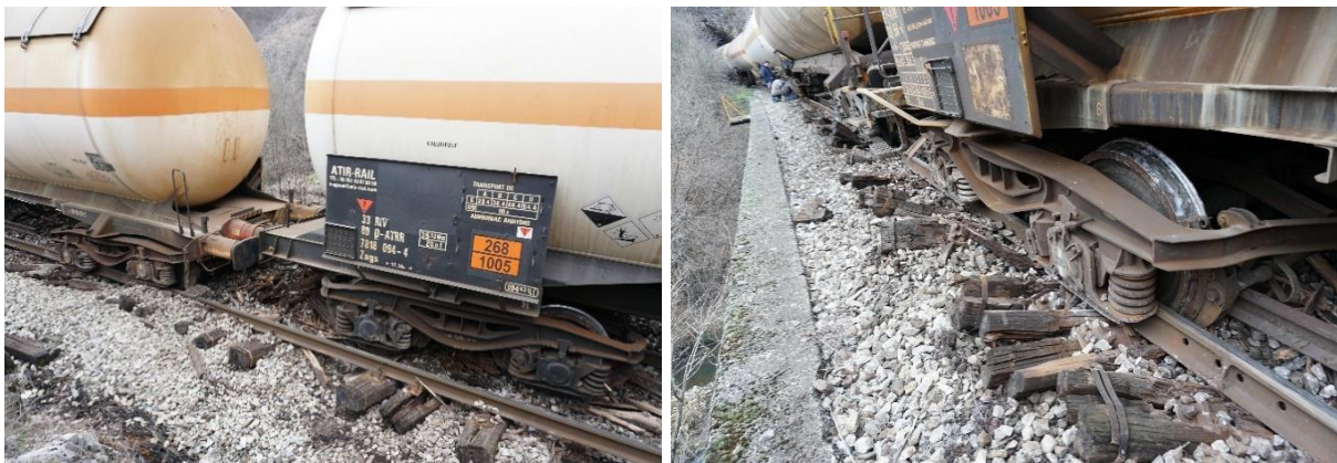
Figure 3.1.4: The appearance of the derailed wagon parts
