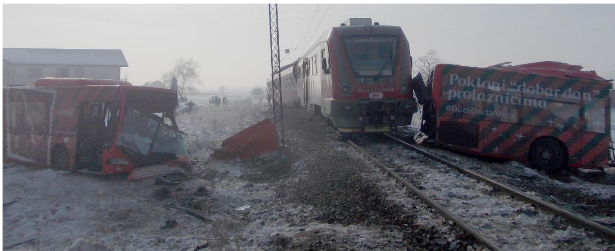
Fig. 4.4.1.1.: The appearance of the vehicle after the serious accident (view in direction to the end of the train)
