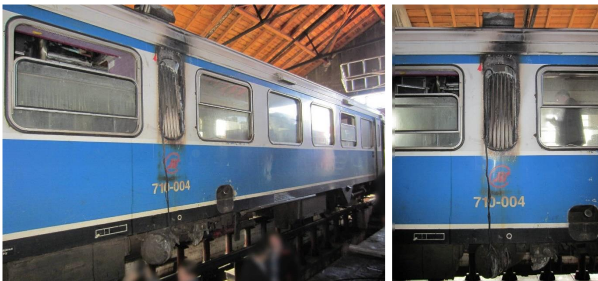
Fig. 4.1.1.1: The appearance of DMK 710-004 on fire (middle part from the outside)
