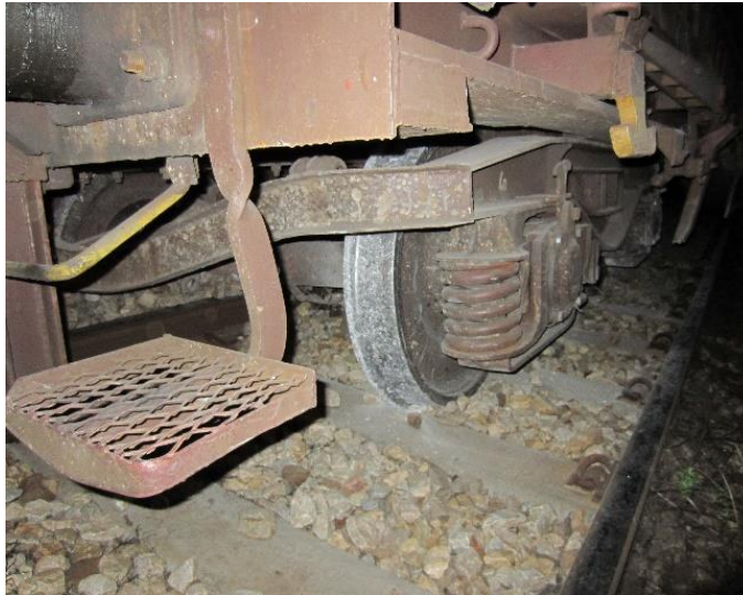
Fig. 3.2.1: Appearance of part of derailed bogie
