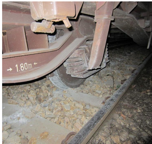
Fig. 4.1.1.2: Appearance of part of derailed bogie
