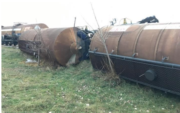
Fig. 3.7.1: Appearance of derailed wagon
