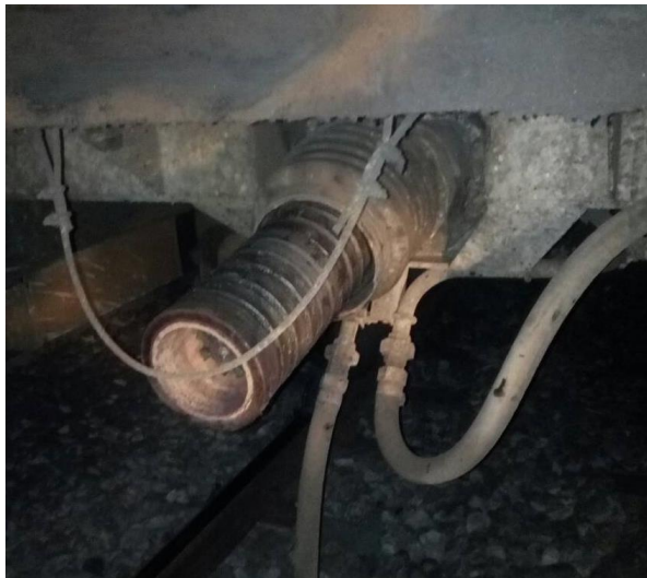
Fig. 3.1.1: Appearance of the part of decoupled clutch on the trailer 416-004
