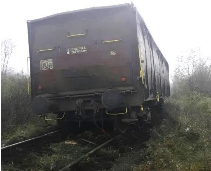
Fig. 3.6.1: Appearance of derailed wagon
