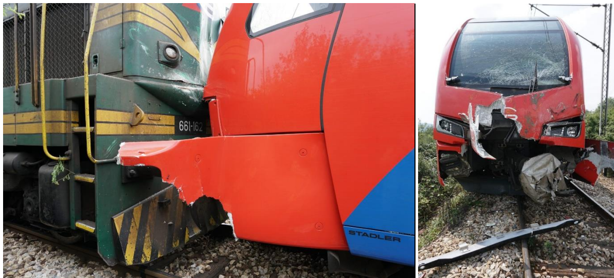
Figure 3.3.1: The appearance of the damage on the railway vehicles after the collision of trains
