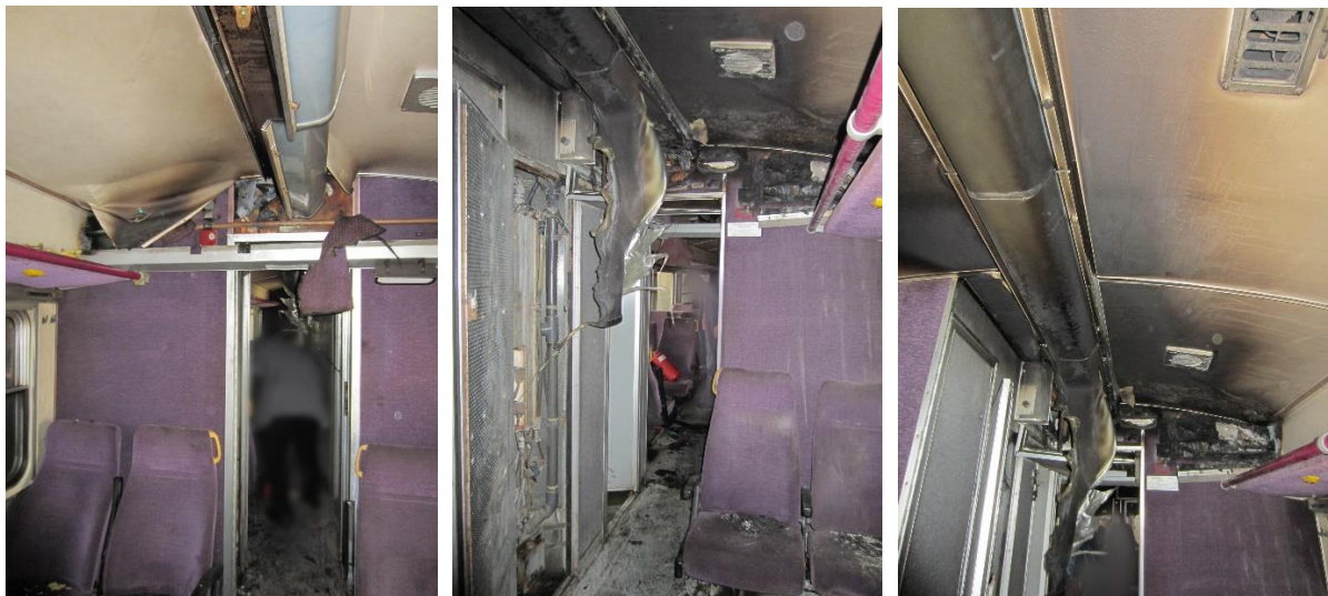
Figure 3.1.2: View on passenger compartment DMK 710-004 on fire
