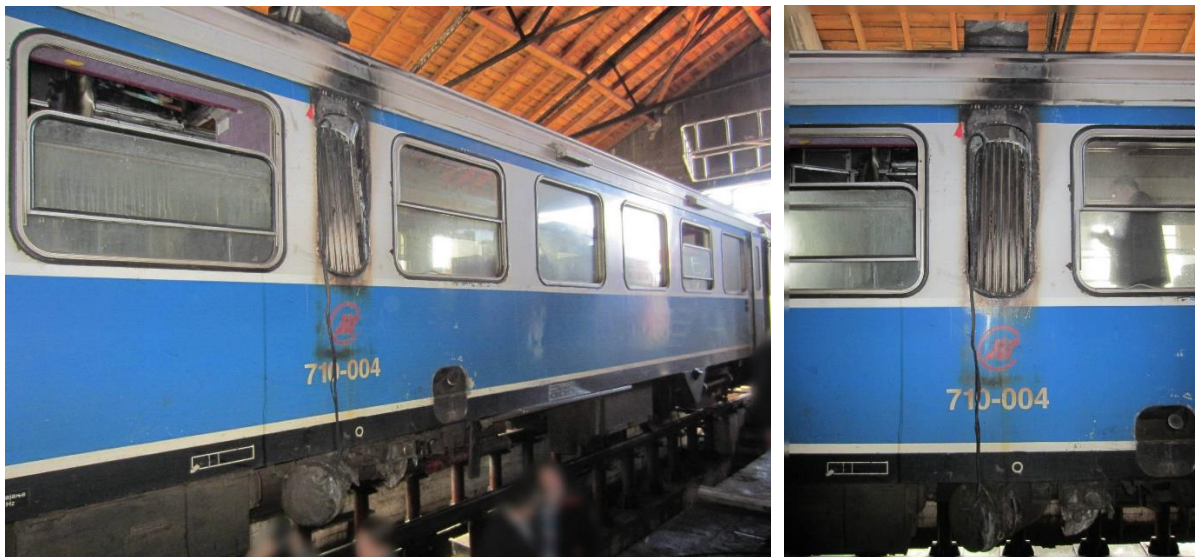
Figure 3.1.1: The appearance of DMK 710-004 caught on fire (middle part from the outside)
