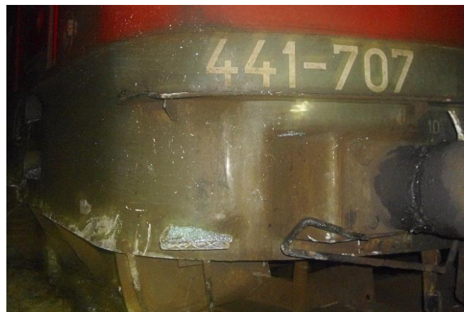
Figure 4.2.1.2: The appearance of the damages on the loc. 441-707
