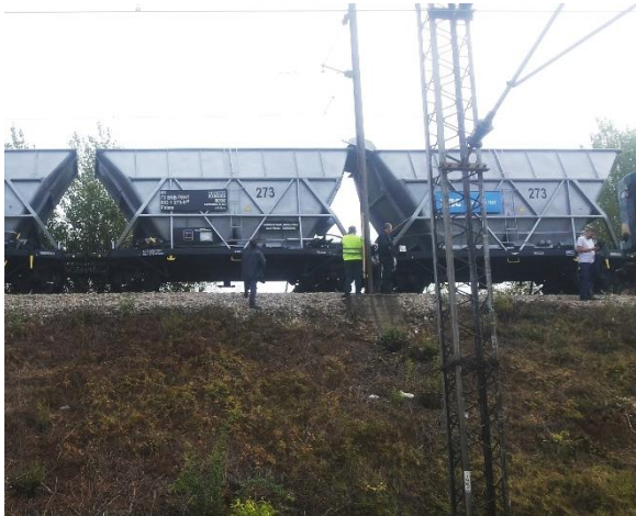
Figure 4.3.1.1: Appearance of the derailed wagon
