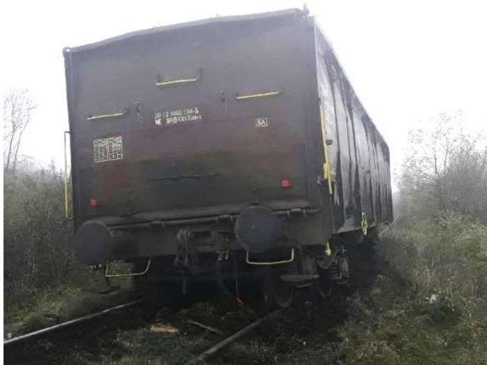
Figure 4.5.1.1: Appearance of the derailed wagon
