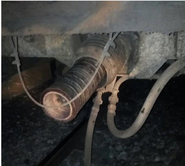
Figure 4.1.1.2: Appearance of a part of the decoupled coupling on the trailer 416-004
